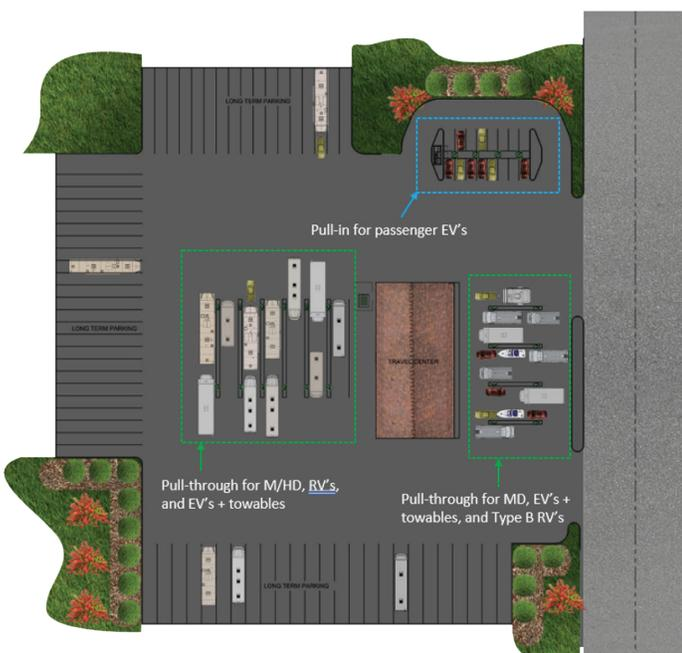
**Figure 4-1 Illustration of Charging Hub with Pull-Through Chargers**
