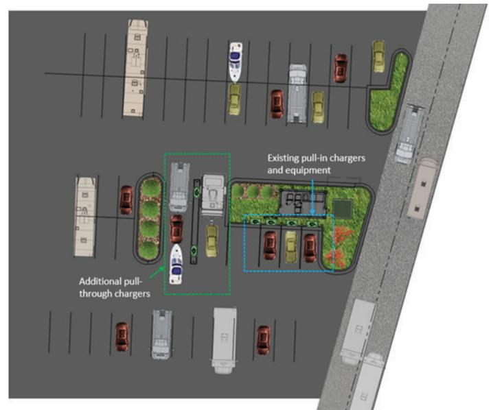
Figure 4-2 Illustration of Retrofitting an Existing EV Charging Site
